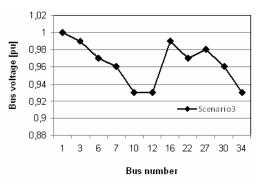
Fig.5. Network bus voltages at scenario 3 when the DG units are controlled by power factor.
