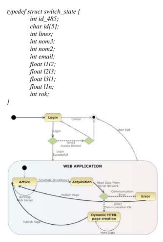
Fig. 4. UML state diagram of the on line monitoring procedure
