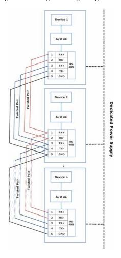
Fig. 2. Acquisition Serial Network
