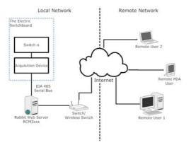
Fig. 1. Overall architecture for the switchboard monitoring prototype
