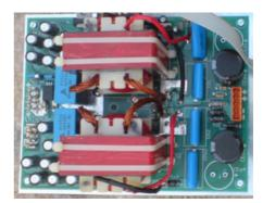
Fig. 9. Top view of the boost high-gain.
