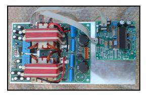
Fig. 8. Boost converter prototype.
