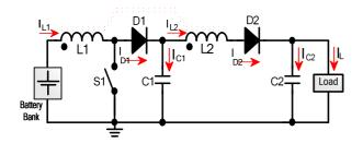
Fig. 7. Electric schematic of the boost converter.
