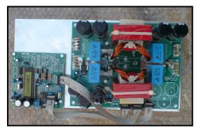
Fig. 6. Battery charger prototype.
