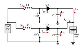
Fig. 5. Basic electric schematic of the battery charger.
