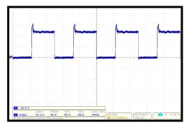
Fig. 10. Voltage across the power switch (with load) (20V/div).
