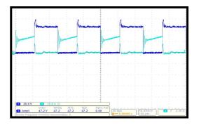
Fig. 11. Current through L1 (CH2) and voltage across the power switch (CH1). (20V/div), (10A/div)
