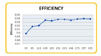
Fig. 15. High gain boost converter efficiency.
