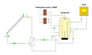
Fig. 5. Scheme of the heating system for domestic water.
