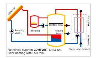
Fig. 4. Operating principle of the solar DHW system.
