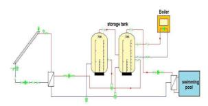
Fig. 3. Scheme of the heating system for .competition pool.
