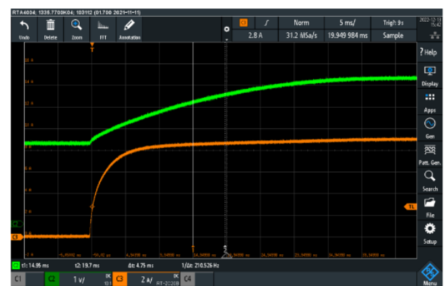
Fig. 7. Commercial PEM electrolyzer measured response to a current step test.
