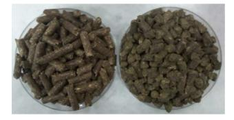
Figure 2. Pellets from olive tree branches and olive tree leaves, respectively.
