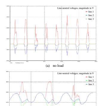
(b) all phases loaded by 12 x 3 kW<sub>p</sub> profiles
