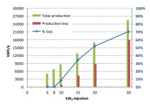
Fig. 8. Yearly production and loss due to overvoltage vs. PV peak power in case of single phase injection at the end of the feeder and all phases loaded by 12 x 3 kW<sub>p</sub> profiles
