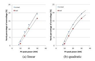
Fig. 7. Yearly percentage of overvoltage vs. PV peak power in case of no load and all phases loaded by 12 x 3 kW<sub>p</sub> profiles
