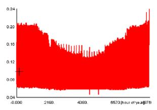
Fig. 3. Residential power consumption during a year, normalized to 1000 p.u. for the yearly total [5].
