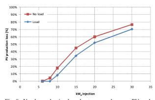
Fig. 9. Yearly production loss due to overvoltage vs. PV peak power in case of load and no load conditions
