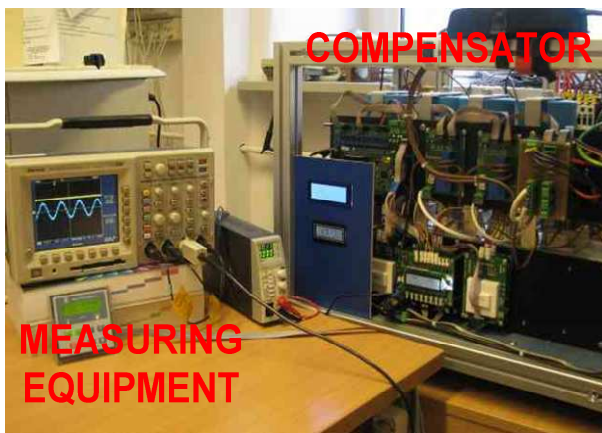
Fig. 10. Power electronics converter with control system based on the DSP processor
