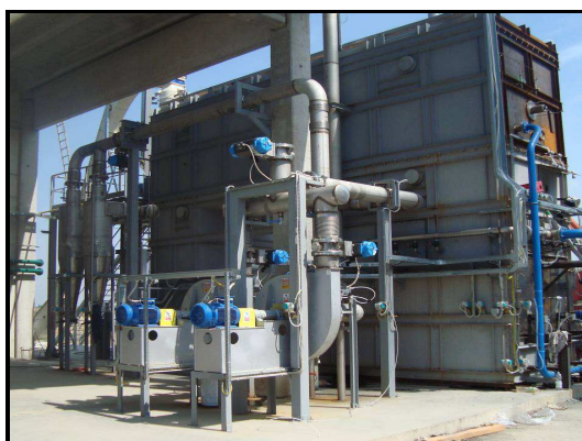
Fig. 1. Overall view of the pyro-gasification unit: main processor with the suction fans and, rearward, the dedusting cyclones.
