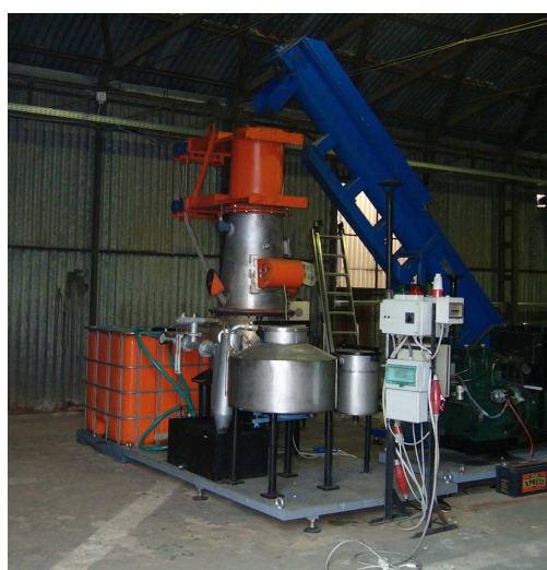
Fig. 4. The Ankur-Caema downdraft gasifier at DIMSET/SCL with gas cleaning equipment and a Fieldmarshal 10 kW el genset.
