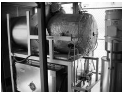
Fig. 1. View of the microturbine tested and its Digital Power Controller (DPC)
