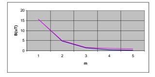
Fig. 6. Magnetic flux density versus distance in the working place neighbor to the secondary bus bars of the transformer substation
