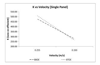
Figure 2: Constant k as a function Velocity [Single Panel]
