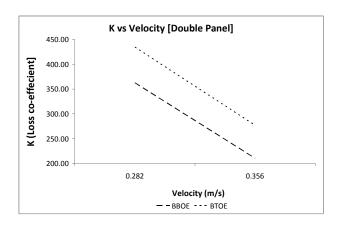
Figure 3: Constant k as a function Velocity [Double Panel]
