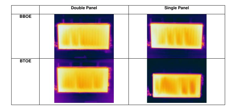
Table 3: Thermal Images for single and double panel radiators in different pipe layout
