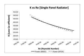
Figure 5: Loss Co-efficient Constant vs Reynolds Number [Single Panel Radiator]
