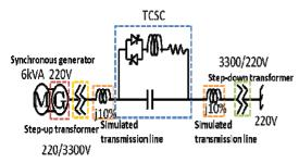
Fig.3. Single machine infinite bus system
