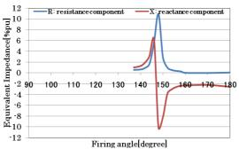
Fig.12 Impedance Characteristic by simulation
