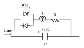
Fig.1. Configuration of TCSC prototype
