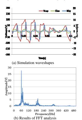
Fig.10 Simulation results at firing angle 136°
