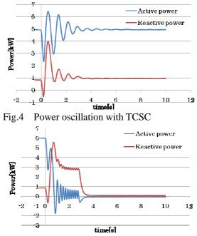
Fig.5 Power oscillation without TCSC
