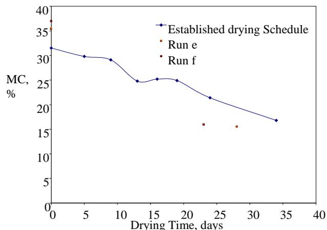
Fig. 4.3. Rainy Season Drying Curve with initial and final moisture contents for commercial drying runs.
