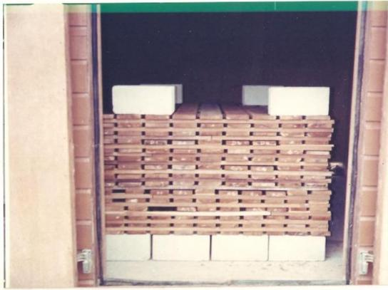
Fig. 3.1. Lumber stacked in the solar kiln timber dryer.
