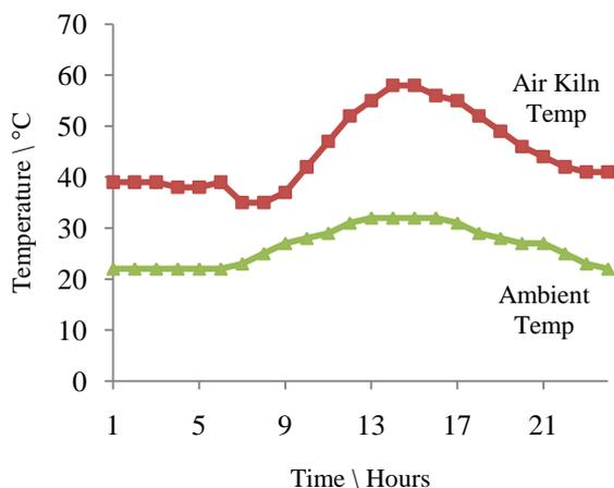
Fig. 4.1. Typical Daily Cycle of Drying Conditions in the Loaded Solar Dryer
