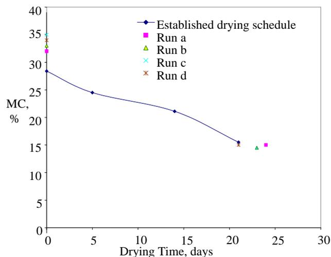
Fig. 4.2. Dry Season Drying Curve with initial and final moisture contents for commercial drying runs
