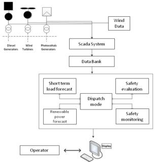
Fig. 1. Main architectural of the supervisory controller.
