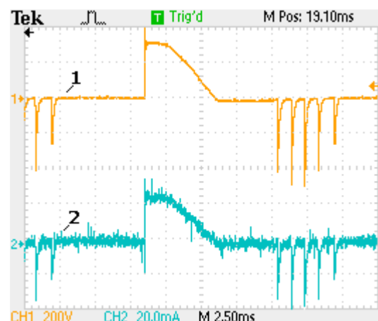
Fig. 7. Voltages and currents for weak load on the triac-based dimmer
