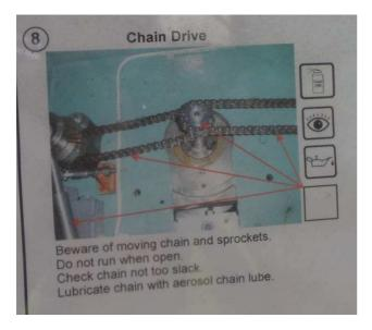
Fig. 4 – Filter line 1 TPM panel – Chain Drive [7]
