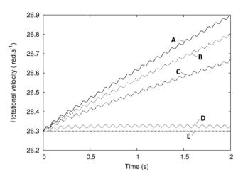
Fig 7. Evolution of the rotational velocity for increasing values of the resistive torque (A-D). The straight dash line (E) represents the target velocity corresponding to the experimental data.
