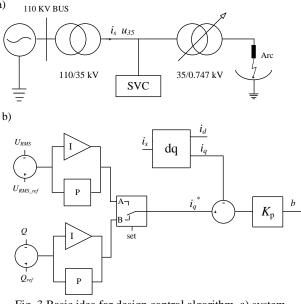
Fig. 3 Basic idea for design control algorithm, a) system configuration; b) control scheme
