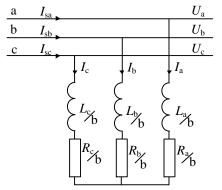
Fig. 2 The simplified equivalent scheme of the TCR
