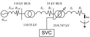
Fig. 3 Single-line scheme of the plant network
