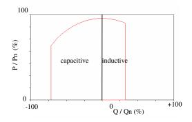
Fig. 12. Possible supplied reactive power of a DFIG
