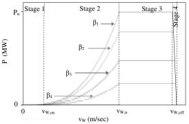
Fig. 3. Power curve of a wind power plant for several  $\beta$  values
