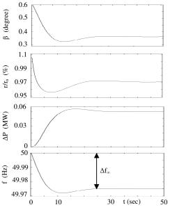
Fig. 6. Primary control with a wind power plant with a DFIG
