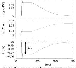
Fig. 10. Primary and secondary control with a wind farm implemented with DFIG
