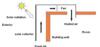
Fig. 1. Solar air collector system schematic
