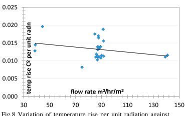
Fig.8 Variation of temperature rise per unit radiation against flow rates.
