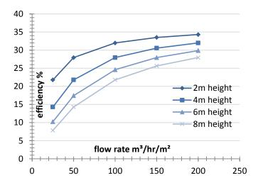
Fig.9 Variation of percentage efficiency against flow rate
