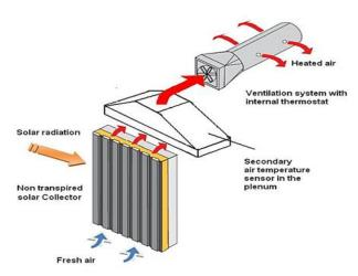
Fig.4. BPSC system schematic
