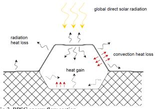
Fig.3. BPSC energy flow section.
