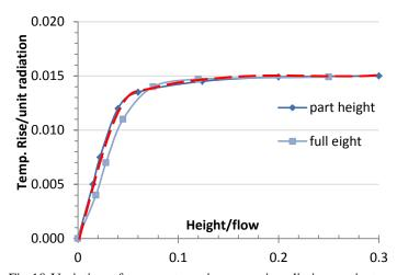
Fig.10 Variation of temperature rise per unit radiation against flow rates
