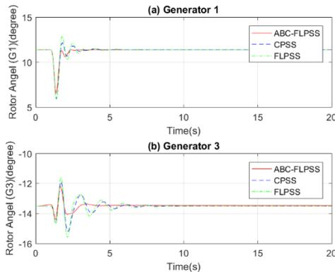
Fig. 11. Transmission Line 1 rotor angles with a three-phase fault
