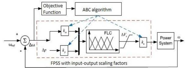
Fig. 4. ABC algorithm for tuning FLPSS input-output scaling factors
