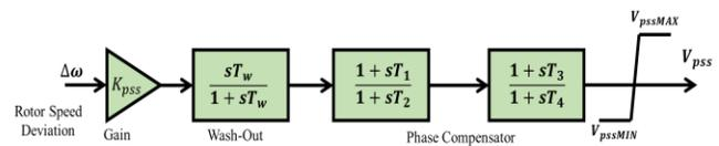
Fig. 2. Conventional Power System Stabilizer Structure
