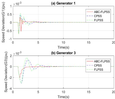
Fig. 10. Transmission Line #1 speed deviations with a three-phase fault
