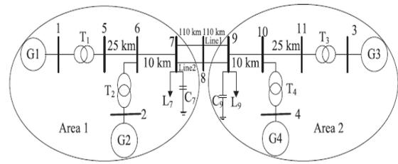
Fig. 1. Two-area, four-machine, eleven-bus test power system
