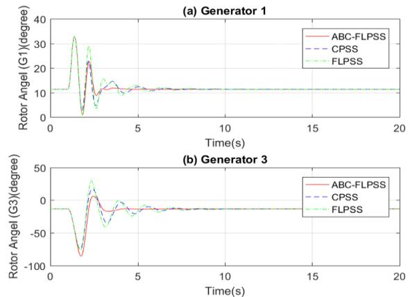
Fig. 8 Generator #1 rotor angles with three-phase fault
