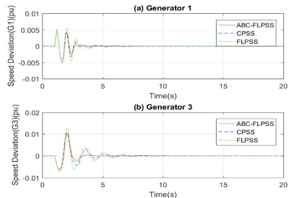
Fig. 7 Generator #1 speed deviations with three-phase faults.
