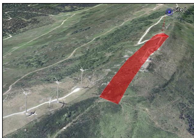
Fig. 3. Aerial view that shows the results of an impact study on a fixed radio link, where Site I is one of the ends of the radio link. Area in red is the set of locations where a turbine would obstruct the link.
