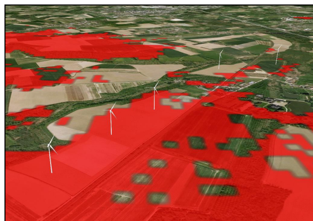
Fig. 1. Constraint mask provided by the algorithms. Area in red is composed by the set of locations where a turbine would degrade the telecommunication service under analysis. Turbines located out of this safeguarding area will not cause degradation.
