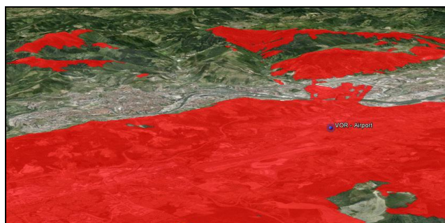
Fig. 4. Aerial views that show the results of an impact study on a radio navigation aid (VOR system). Area in red is the set of locations where a turbine would interfere in the restricted volume for the proper working of the system.
