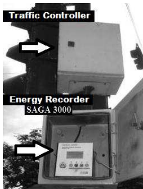
Fig. 4. Measurements made at pedestrian lights with LEDs after replacing.
