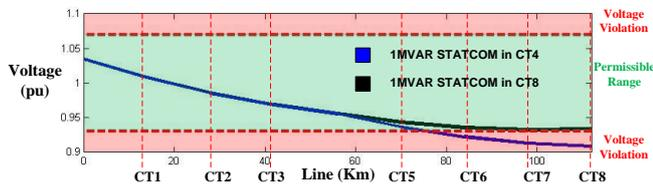
Fig 15. Voltage profile of the selected scenario with OLTC and STATCOM
