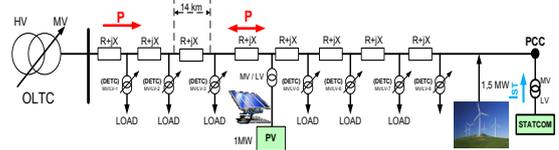
Fig 24. Selected scenario with OLTC, STATCOM and DG
