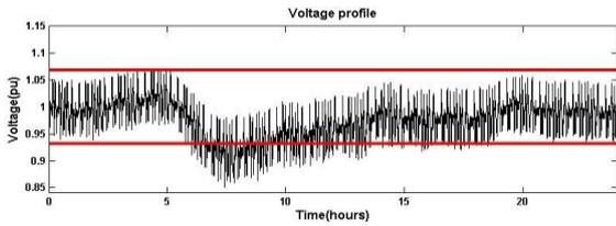
Fig 20. Voltage profile (CT8) of the scenario of Fig 16
