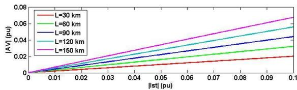
Fig 13.  $|\Delta V|$  in function of the current of the STATCOM
