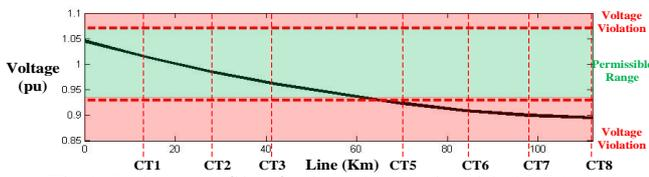
Fig 6. Voltage profile of selected scenario with OLTC
