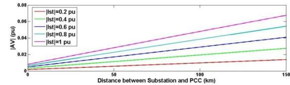
Fig 14.  $|\Delta V|$  in function of the distance PCC-substation
