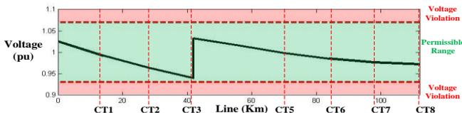
Fig 8. Voltage profile of selected scenario with OLTC and SVR
