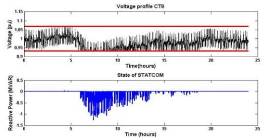
Fig 25. Voltage profile of CT8 and Q-STATCOM
