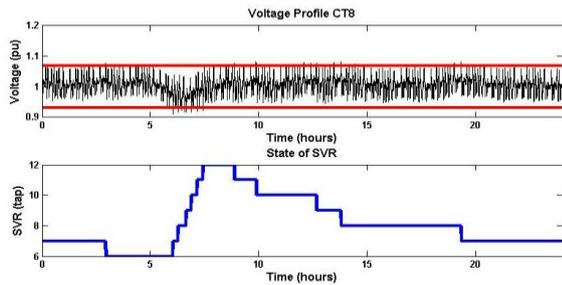
Fig 23. Voltage profile of CT8 and the state of the SVR
