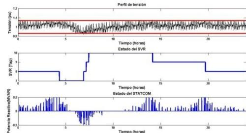
Fig 27. Voltage profile of CT8, state of SVR and Q-STATCOM
