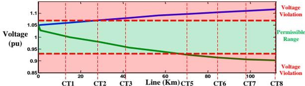
Fig 21. Voltage profile of CT8 and the state of the STATCOM
