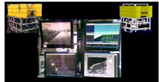
Fig. 12. Control Cabin: comparison of views from real and virtual pilot cameras
