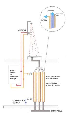
Fig. 2. Swimming pool shower heat exchanger (HX) system.
