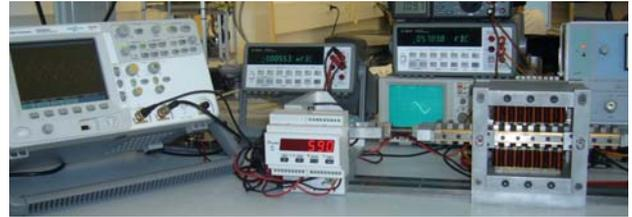
Fig. 6. View of the test setup and of the double-sided LSRM
