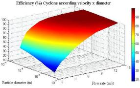
Figure 3 - 3D graph – Efficiency of the cyclones due speed x diameter particles.
