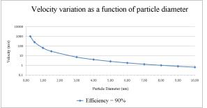
Figure 4 - Speed in function of particle diameter for efficiency in 90%.
