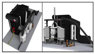
Fig. 3. 3D-Model of twin gasifier, combustor and boiler.
