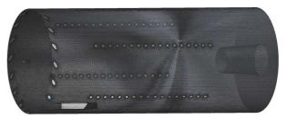
Fig. 4. 2.2 Mio. optimised meshing of the combustor (ICEM).
