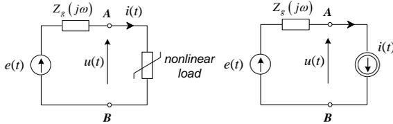
Fig. 1. Mechanism of harmonic proliferation into the network
