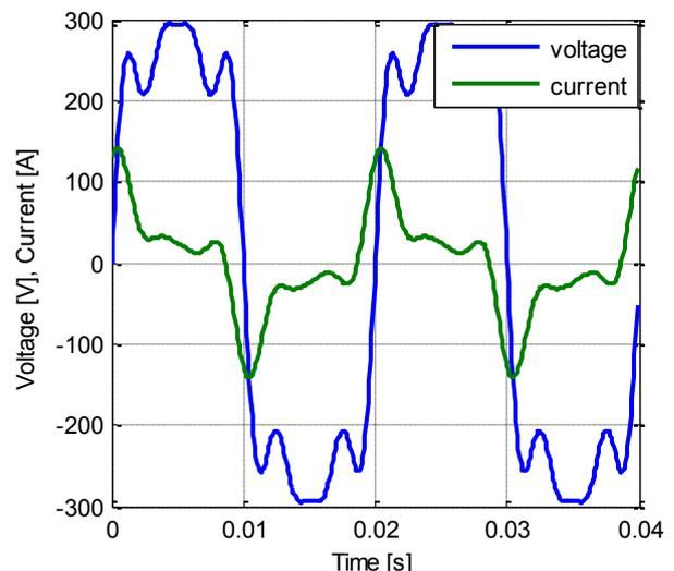
Fig. 3. Simulated current and voltage waveform
