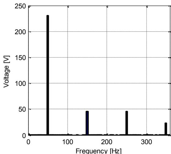
Fig. 4. Spectral components in the voltage
