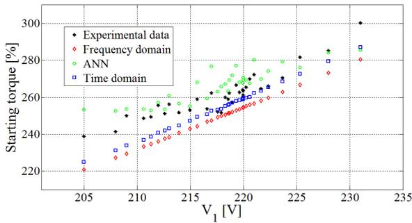
Fig. 3 – Starting torque in relation to  $V_1$
