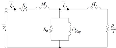
Figure 4. Positive sequence equivalent circuit.
