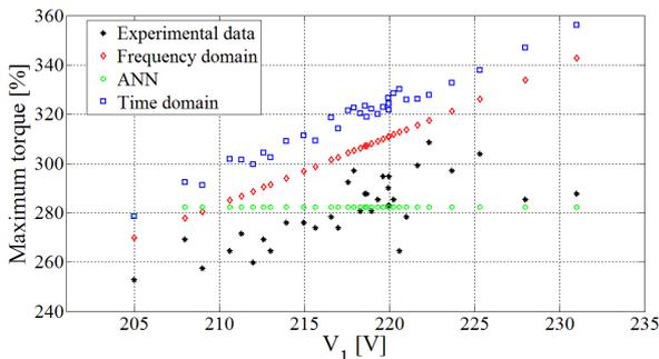
Fig. 4 – Maximum torque in relation to  $V_1$
