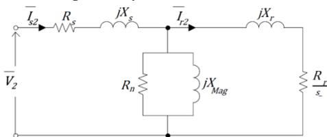
Figure 5. Negative sequence equivalent circuit
