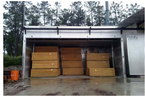
Fig. 1. General view of the greenhouse used for the pine wood heat treatments.
