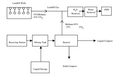
Fig. 2. The Biogas Plant in Jordan.
