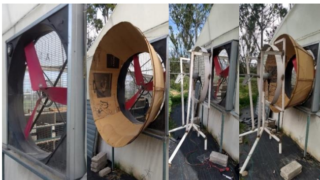
Fig. 2. Experimental tests of an extractor and wind turbine.
