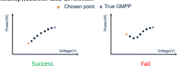
Figure 8 Illustration of success and failure criteria for propose fast GMPPT method
