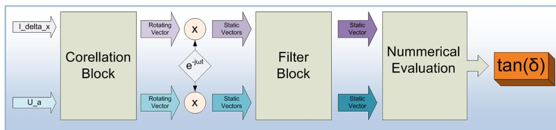
Fig. 3: Loss factor measurement algorithm
