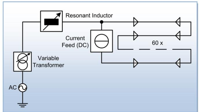
Fig. 1: Simplified structure of the ICAAS
