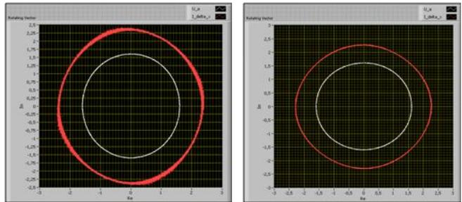
Fig. 4: One step in the process of determining the  $\tan(\delta)$  value: rotating vectors of the voltage  $U_a$  and current  $I_{\delta}$  of a pre-aged cable (left) and a new cable sample (right)
