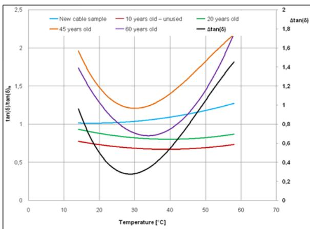
Fig. 5: Dependency of the dissipation factor on the temperature for different cable samples
