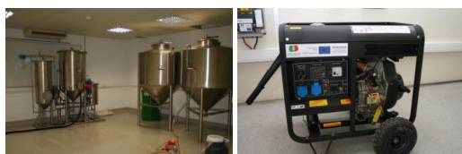
Fig. 13. Production unit of biodiesel (left) and electric generator.
