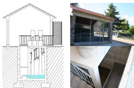
Fig. 4. Cross-section and perspective photos of the pico hydro power house.
