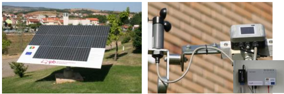
Fig. 11. Solar tracker (left) and sensors (right) for remote monitoring.
