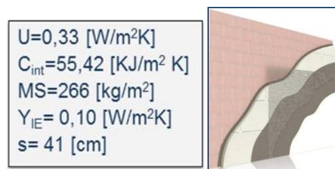
Fig. 5 : External thermal insulation system.
