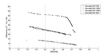
Figure 2. Efficiency of the solutions as a function of overall illuminance uniformity in a one sided configuration. HPS means high pressure sodium and HPM, high pressure mercury.
