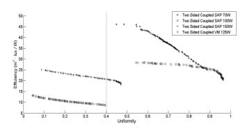
Figure 3. Efficiency of the solutions as a function of overall illuminance uniformity in a two sided coupled configuration. HPS means high pressure sodium and HPM, high pressure mercury.
