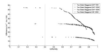
Figure 4. Efficiency of the solutions as a function of overall illuminance uniformity in a two sided staggered configuration. HPS means high pressure sodium and HPM, high pressure mercury.
