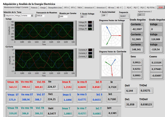
Fig. 15. Experimental test under a sinusoidal and balanced three-phase system connected to three phase transformer a load without.
