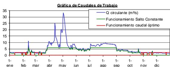
Figure. 11 Comparison of work flow to operate at constant head vs. optimum flow rate; year 2007 (average year).
