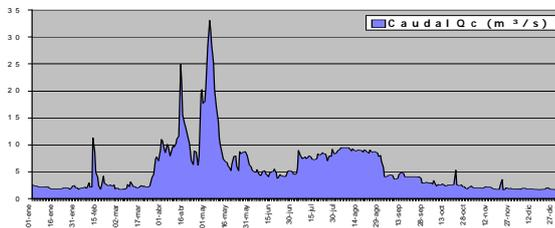
Fig. 2a Circulating flows in the Iregua river for an average year (2007). Source (CHE, Confederación hidrológica del Ebro, Ebro hydrological confederation).
