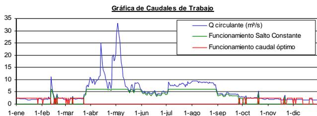
Fig.5 Comparison of work flow to operate at constant head vs. Optimal flow in 2007 (average year) Francis turbine spiral case.
