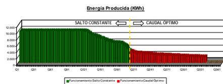
Figure 10. Classified produced energy for a power station equipped with Francis turbine of open chamber (average year).
