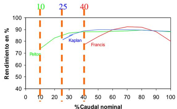
Fig. 1 Performance characteristic of different turbine types, applied the technical minimum flow.
