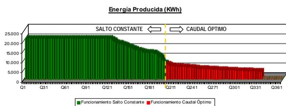
Figure 6. Classified produced energy for a power station equipped with Francis turbine of spiral chamber(average year).
