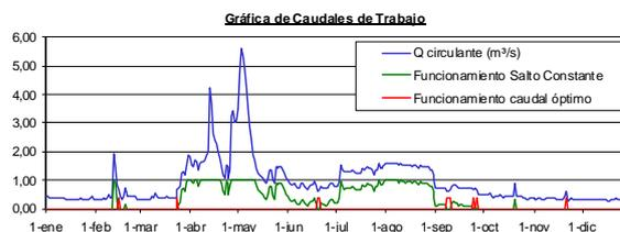
Fig. 7 Representation of work flow with constant head operation in 2007 (average year). Pelton turbine.
