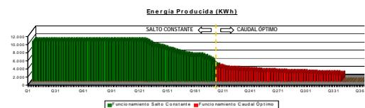
Figure 12. Classified produced energy for a power station equipped with Kaplan turbine (average year).
