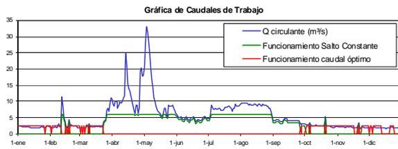
Fig. 9 Comparison of working flow to operate at constant head vs. Optimum flow. 2007 (average year).
