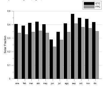
Fig. 3. Monthly solar fraction contributed - FPC vs ETC
