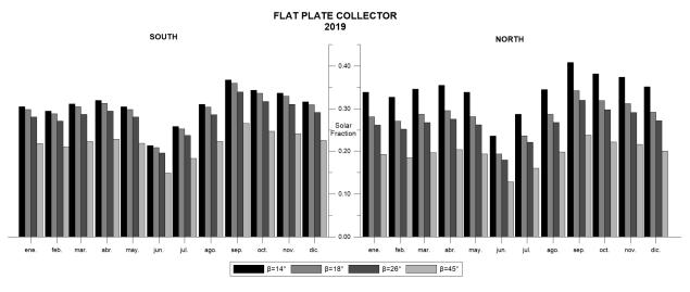
Fig. 1. Solar thermal fraction in the city of Cuenca - Ecuador according to FPC with typical roofs slopes
