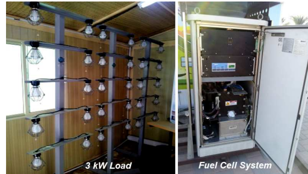
Fig. 8 ElectraGen™ fuel cell system and the 3kW load
