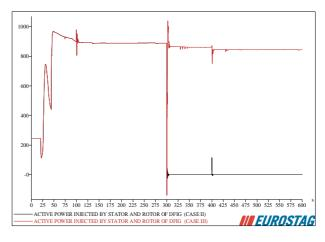
Fig. 8. Active power injected by stator and rotor of DFIG.
