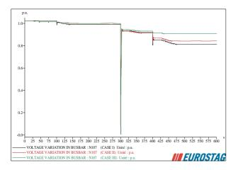
Fig. 10. Voltage variation in busbar 107.
