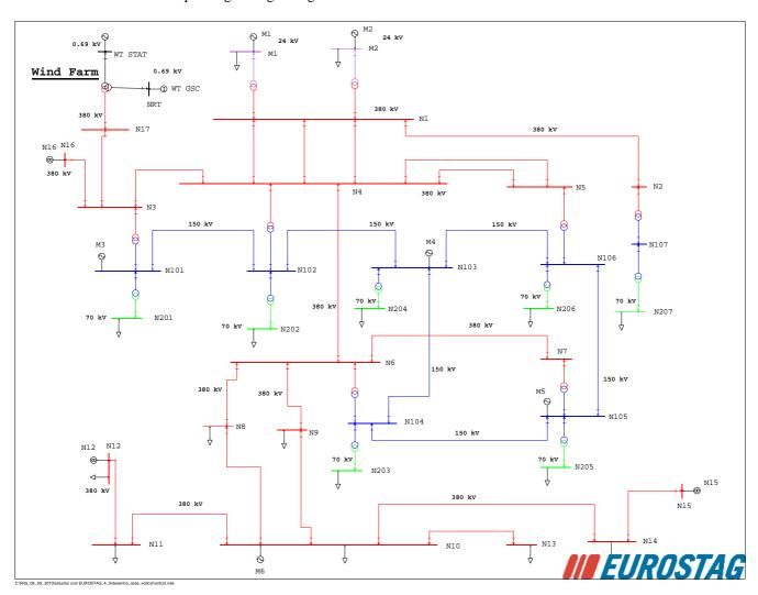
Fig. 4. Cigré test power network single line diagram [9], [10].
