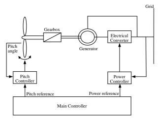
Fig. 2. Model of the DFIG scheme [6].
