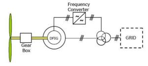
Fig. 1. Wind Turbine with DFIG.
