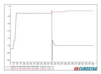
Fig. 7. Speed of the induction machine.
