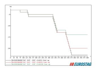
Fig. 12. Under Load Tap Changers position.
