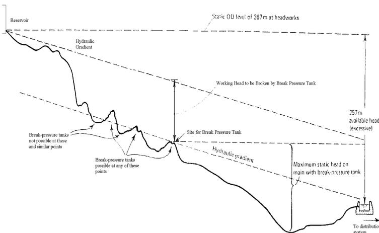
Fig.1 Typical scenario where break pressure tank becomes necessary (Gray, 2010)
