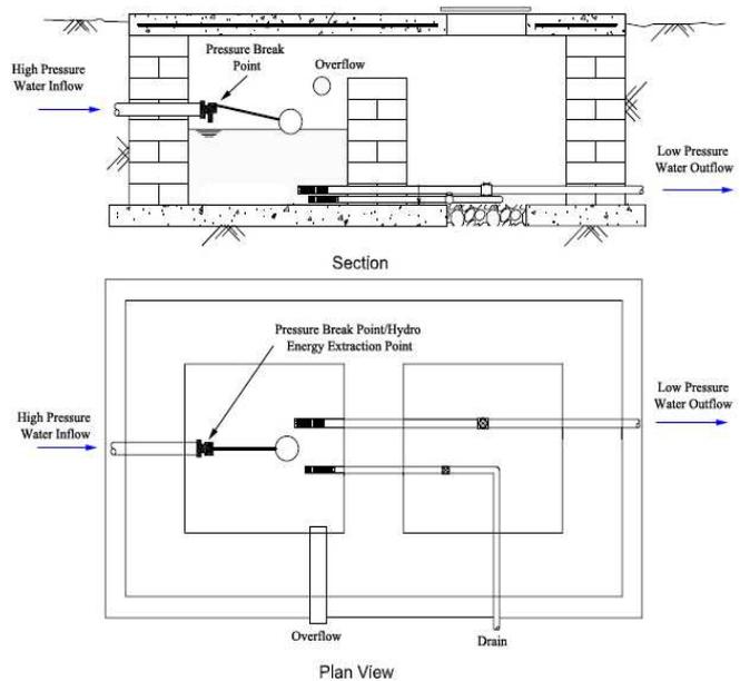
Fig.2 Typical Break Pressure Tank
