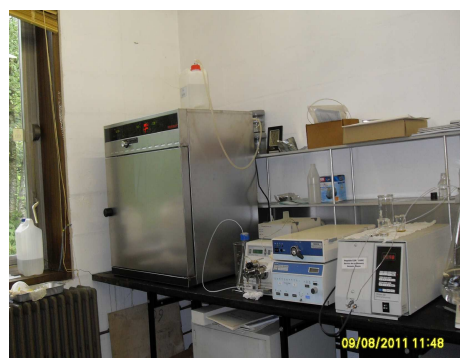
Fig. 2. Conditioning Drying Oven
