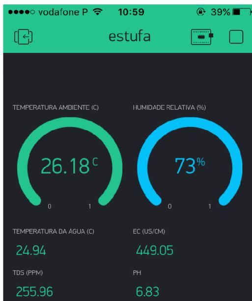
Fig. 9. Blynk graphical interface on smartphone.
