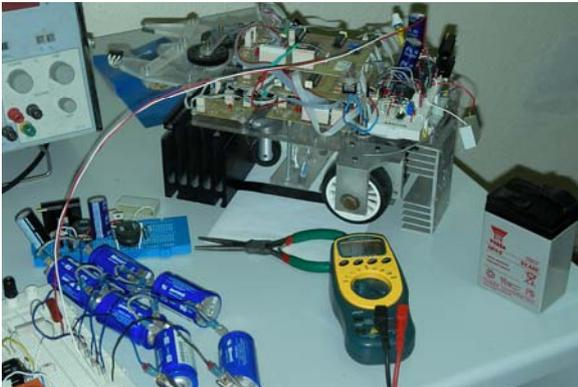
**Figure 4.** Mobile robot prototype together with the new supply system formed by ultracapacitors + SEPIC converter.
