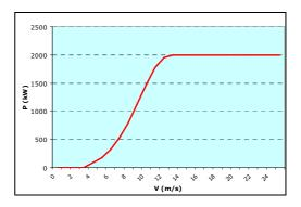
Figure 7. 2 MW Wind turbine power curve.
